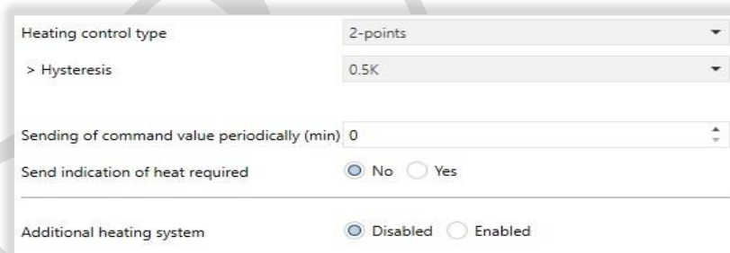
Fig 24 : Heating 2-Points Control Configuration
